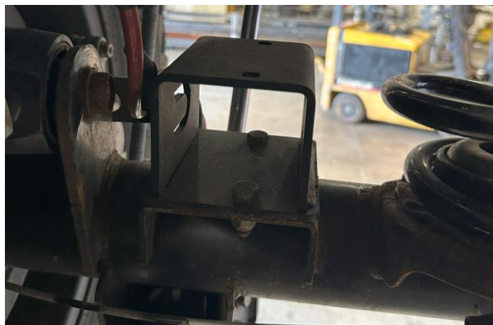
Figure 1: Extension located on bump stop perch with bolts dropped in holes
