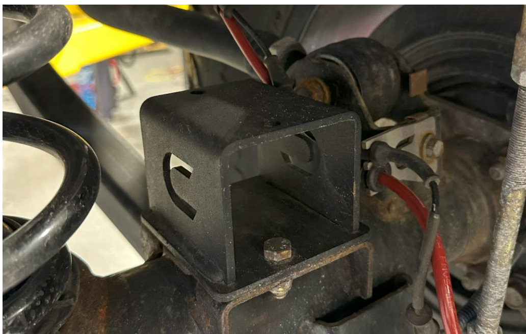
Figure 2: Bump stop installed with supplied hardware
