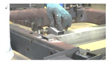
Following proper welding procedures, tac weld your rear shock mount onto the frame before welding it on fully. Weld 100% around all edges.
