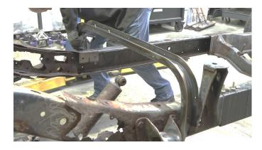
Once in place, use a 15mm socket and 14mm wrench to reinstall the hardware.
