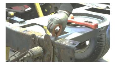
Then, tighten your hardware with a 14mm socket and a 15mm wrench.
