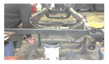
Then, tac weld your crossmember into place before welding it on fully. Weld 100% around all edges.
