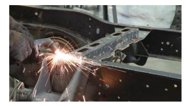
After cutting out the rivets, punch them out with a hole punch. Repeat on both sides.
