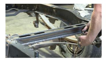
Then, screw in the eight remaining 30mm screws on the top of your frame rail. Tighten them with a 15mm socket and 14mm wrench.
