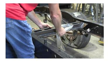
Once you have them aligned, screw in the eight included 25mm screws where the support plate and crossmember meet.
