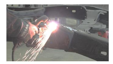
Grind the frame free of rust and debris, revealing bare metal.
