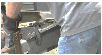
Following proper welding procedures, tac weld the leaf spring frame section onto the frame before welding the part on fully. Weld 100% around all edges.
