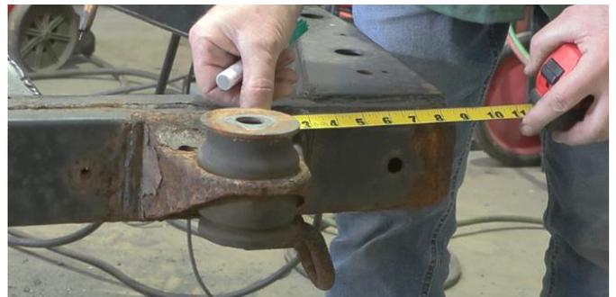
Using the measurements you took on the opposite side of the frame, mark where the center will be with a paint marker.
