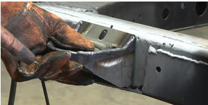
Remove any potential fire hazards from the work area. Following proper welding procedures, tack weld the part onto the frame before welding the part on fully. Weld 100% around all edges.
