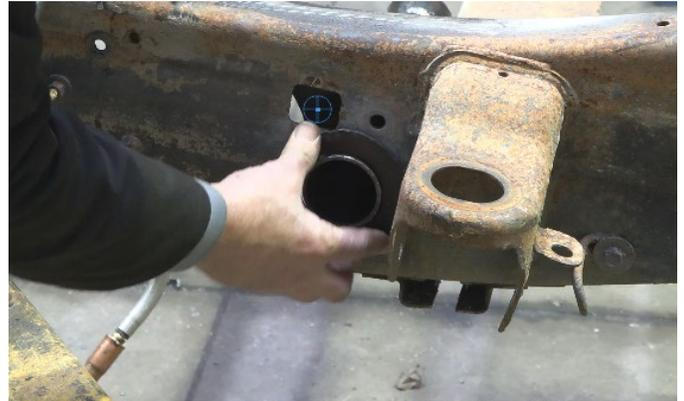
Completely weld the plate around the outside in inner edges.
