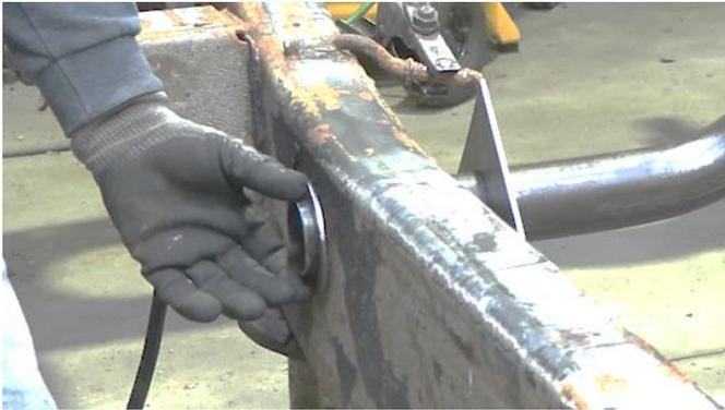
Following proper welding procedures, tack weld your driveshaft crossmember onto the frame before welding it on fully. Weld 100% around all edges.
