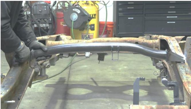
Once you have your crossmember in place, take the included hardware and screw them into place where your rivets were originally located. Then, tighten your hardware with a 14mm socket and 15mm wrench.
