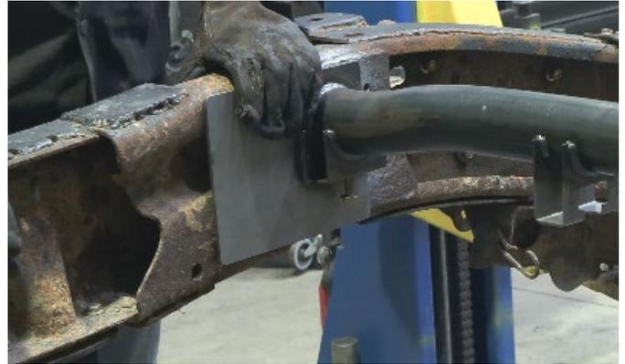
Tac weld the pre-welded side into place and verify its alignment. Align the opposite side's plate with the top of the frame rail and tac weld it into place.
