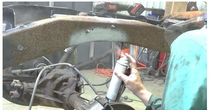
Our part features a perforated plate that can be removed to fit over your existing bolts. If you decide not to remove the bolts, cut out the perforated plates on the top and bottom of your frame section.
