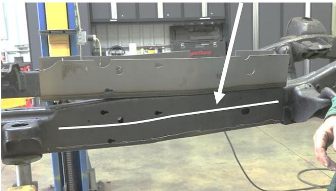
Our part features a perforated plate to fit over your existing crossmember. To do this, bend over the two plates. You may need to relieve the plates slightly to make them easier to bend over.
