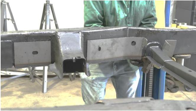
Use a wrench to bend the plates against the frame located above the crossmember.
