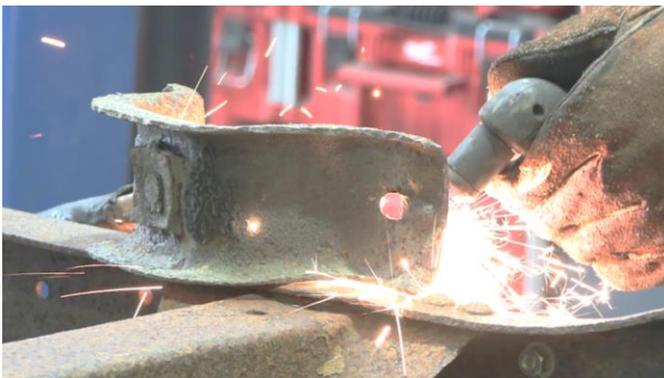
Hold the part up to the frame and mark off its coverage.
