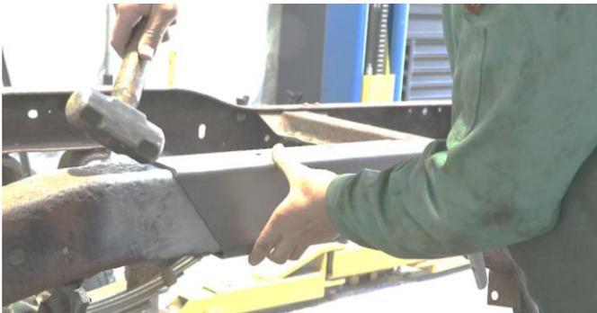
Following proper welding procedures, tack weld the over-axle frame section to the frame before welding the part on fully. Weld 100% around all edges.
