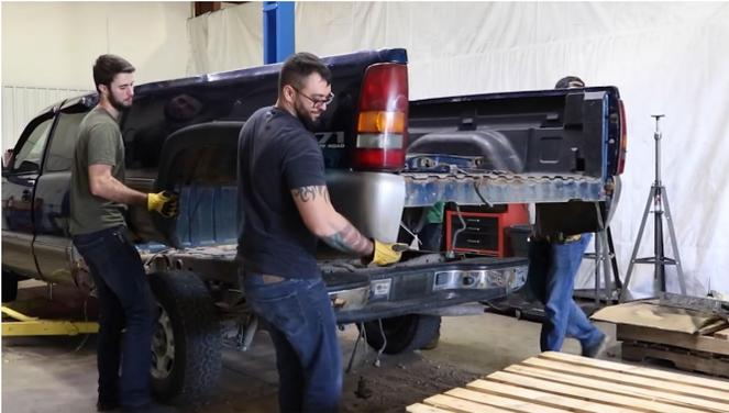
Cut off the 4 rivets retaining the part, followed by punching out the remaining material with an air hammer. Remove the crossmember.
