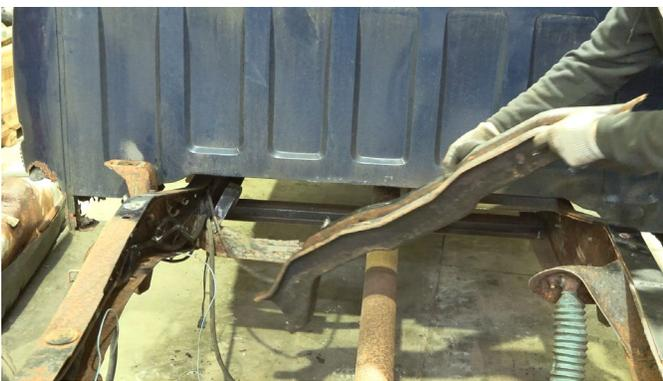
Clean and grind the area free of rust and debris, revealing bare metal. Coat the area with a primer to help prevent against further rust development.
