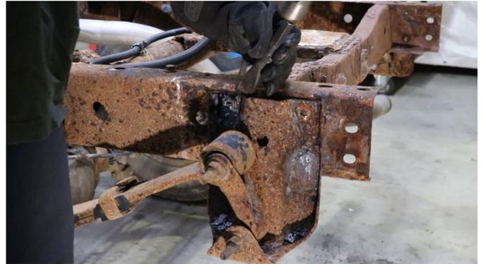
Begin cleaning the area free of rust and debris, revealing bare metal.
