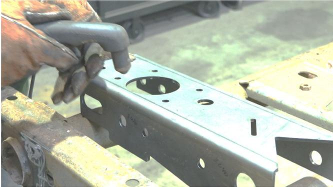
Hold the center frame section up to the frame making sure the frame holes align. If they do, insert two bolts to secure the component in a fixed position.
