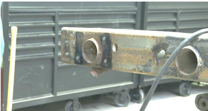
Additionally, grind the frame rails free of rust to expose the bare metal where your repair section will be installed.
