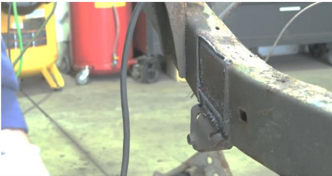
Grind the frame free of rust and debris, revealing bare metal.
