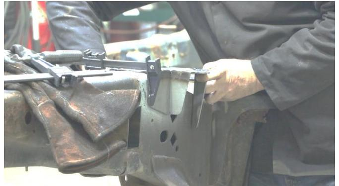
After securing your part, take your tape measure and using the part on the opposite side of your vehicle, measure the distance between the top of the frame rail and the top of your part.
