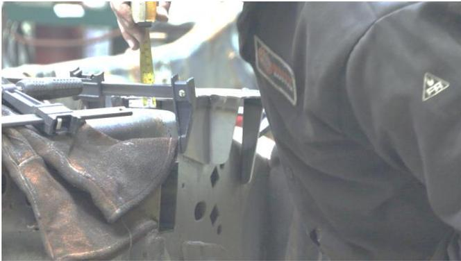
Following proper welding procedures, tack weld your front bed mount onto the frame before welding it on fully. Weld 100% around all edges.
