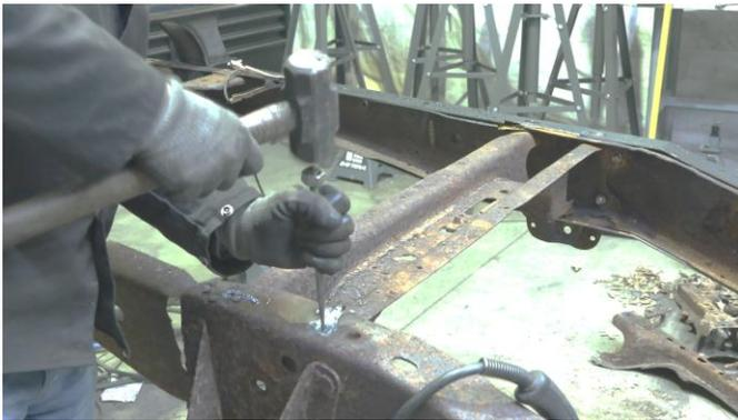
After removing the rivets, remove your crossmember. You can cut the crossmember in half to make it easier to remove.
