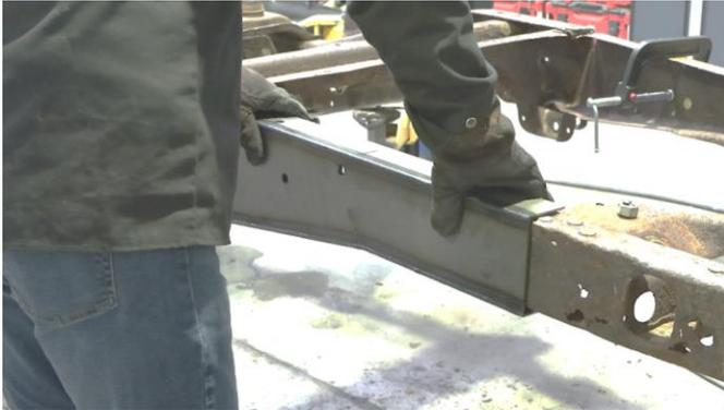
Following proper welding procedures, tack weld your over-axle frame section onto the frame before welding it on fully. Weld 100% around all edges.
