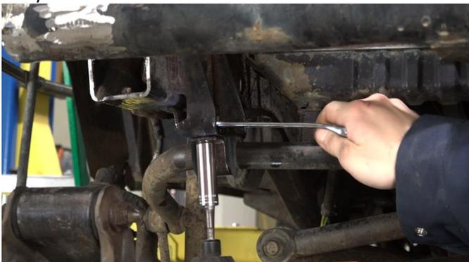
Place the part over the front cross member and take note of its measurements. Draw a line around the frame rail where the part ends. **NOTE: The following steps require accurate measurements in order to allow correct amounts of weld-able frame.**
