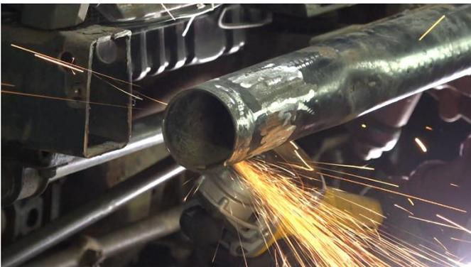
Cut away the section just inside the markings, while **avoiding damage** to the sway bar bracket. This will
