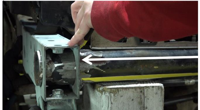
Take note of any difficulties and cut away any obstructions. The part may fit snugly and require force. If you have to bend the front cross member to fit the part into place, you may need to remove very small increments of material from the frame rail until it is flush. **NOTE: Removing too much**
