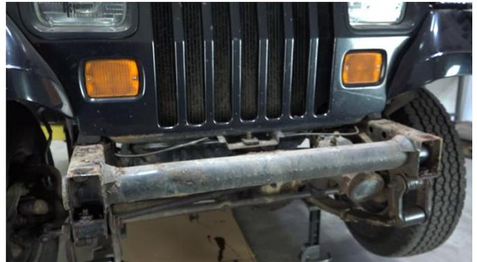
Using a T55 Torx, remove the front bumper, frame cover, and with a 10mm socket remove the cover support bracket.
