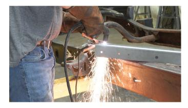
Hold the part up to the frame and mark off its coverage. Ensure you remove any lines or power harnesses from the work area before continuing.
