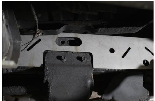
(OPTIONAL): Coat the part with a weld-able primer or other rust inhibitor prior to installation to help prevent or reduce the risk of rust formation.
