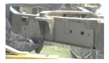
Following proper welding procedures, tac weld your mid frame section onto the frame before welding it on fully. Weld 100% around all edges.
