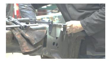
After securing your part, take your tape measure and using the part on the opposite side of your vehicle, measure the distance between the top of the frame rail and the top of your part.
