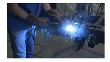
Followed by pushing the rear section up and aligning that area's frame holes, and tac welding it.
