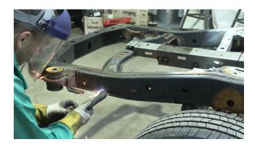
Then, grind down the zones free of rust and debris, revealing bare metal.
