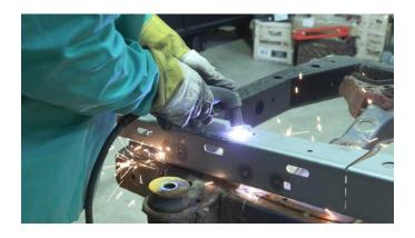
Hold the part up to the frame and mark off its coverage. Bend the opening on your rear frame section to create the contour of your frame. Then, mark your cutline ¾ inch above the bottom of the frame.
