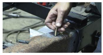
Once all the hardware is in, secure the 4 bolts with a 14mm socket, and nuts with a 15mm socket.
