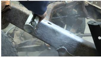
Referencing the mounts on the opposite side of the vehicle, measure 12¾ inches from bolt hole center to center and 3 inches up from the top of the frame, and mark off the install location.
