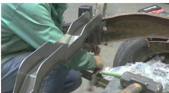
Reinstall the center bolt with a 14mm socket.
