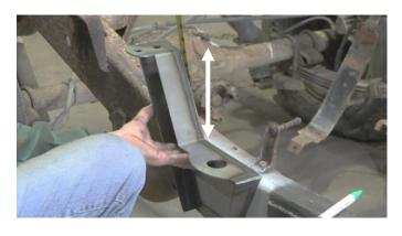
Use your measurements to align your body mount up with the opposite side. Once aligned, mark off its coverage using a paint marker.
