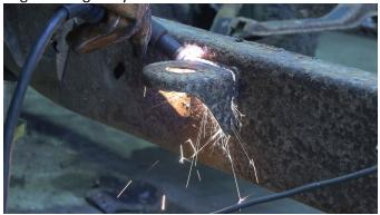
Grind the frame rail free of rust and debris, revealing bare metal.
