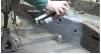
Slide the part onto the frame while using the frame holes or cab mount to help with alignment.
