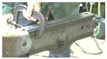
Following proper welding procedures, tac weld the part into place before welding it on fully. Weld 100% around all edges.
