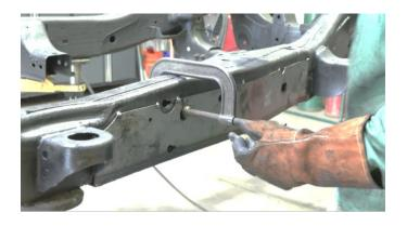
Once in place, weld your part on fully. Weld 100% around all edges.
