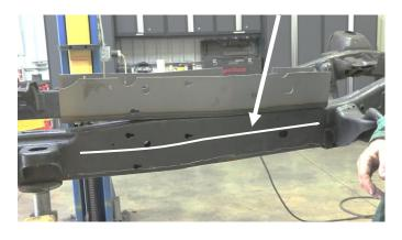
Our part features a perforated plate to fit over your existing crossmember. To do this, bend over the two plates. You may need to relieve the plates slightly to make them easier to bend over.
