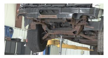
Using a screw driver, push off the shown tabs and remove the break lines.
