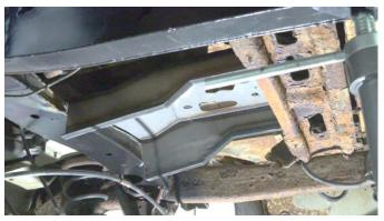
Following proper welding procedures, tac weld the part into place before welding it on fully.
