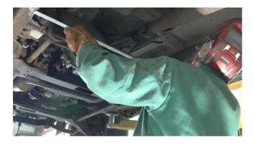
Remove any potential fire hazards from the work area. Following proper welding procedures, tack weld the part onto the frame before welding it on fully. Weld 100% around all edges.
