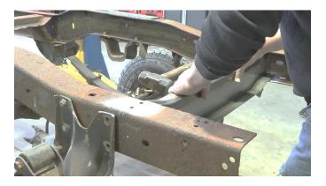
With a 14mm socket and 15mm wrench, screw in the included nuts and bolts on each end of the crossmember.
