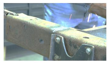
Punch out the remaining rivets using a hole punch.
