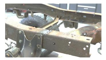
Spray the work area with a weld through primer to help prevent against rust development.
