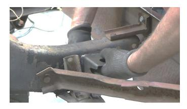
On the bottom of your core support mount, use a 15mm socket to screw in the two 25mm bolts and nuts.
