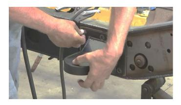
Following proper welding procedures, tac weld the front end of your frame section onto the frame, leaving the side with your body mount loose.
