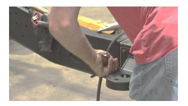
Weld the part on fully. 100% around all edges.
