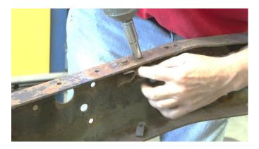
With a 15mm socket, remove the brake line bracket.
