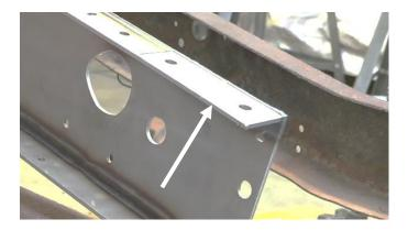
If you decide not to remove this plate, use a 16mm socket and wrench to remove the bolts retaining the transmission crossmember.
