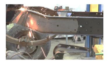
Once in place, weld the parts on fully. Weld 100% around all edges.
