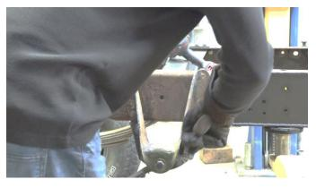
Our part features eight perforated plates on the top and bottom of your frame section to fit over the rivets retaining the factory center frame crossmember. If you decide to keep your rivets, cut out the perforated plates.
