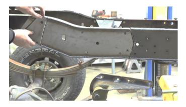
Following proper welding procedures, tac weld your leaf spring frame section and support plate onto the frame.
