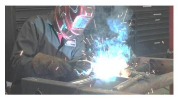
Our part features eight support plates to fit on the top and bottom of your inner brackets located on each end of your crossmember. Hold the plates up to the frame and tac them into place.
