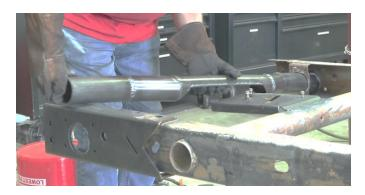
Following proper welding procedures, tac weld the crossmember to the spare tire plate before welding it on fully.
