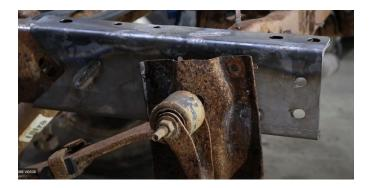
After the rear spring hanger has been reattached to the frame, begin reinstalling the rear shock to the rear spring hanger.
