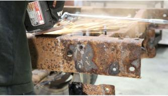
Coat the part and work area in a weldable primer to help prevent future rust and corrosion to the frame.
