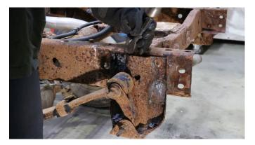
Once you have freed the rear spring hanger from the rear frame section, the two components should separate from each other providing unrestricted access to the area needed for the frame replacement.
