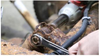
After the shock has been disconnected, begin removing your rear spring hanger with your cutting wheel or torch by cutting off and prying out its rivets.
