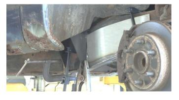
Following proper welding procedures, tac weld the part onto the frame before welding it on fully. Weld 100% around all edges.
