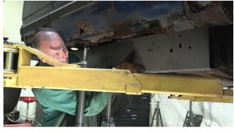
Tac-weld the part and confirm its alignment before completely welding it onto the frame.
